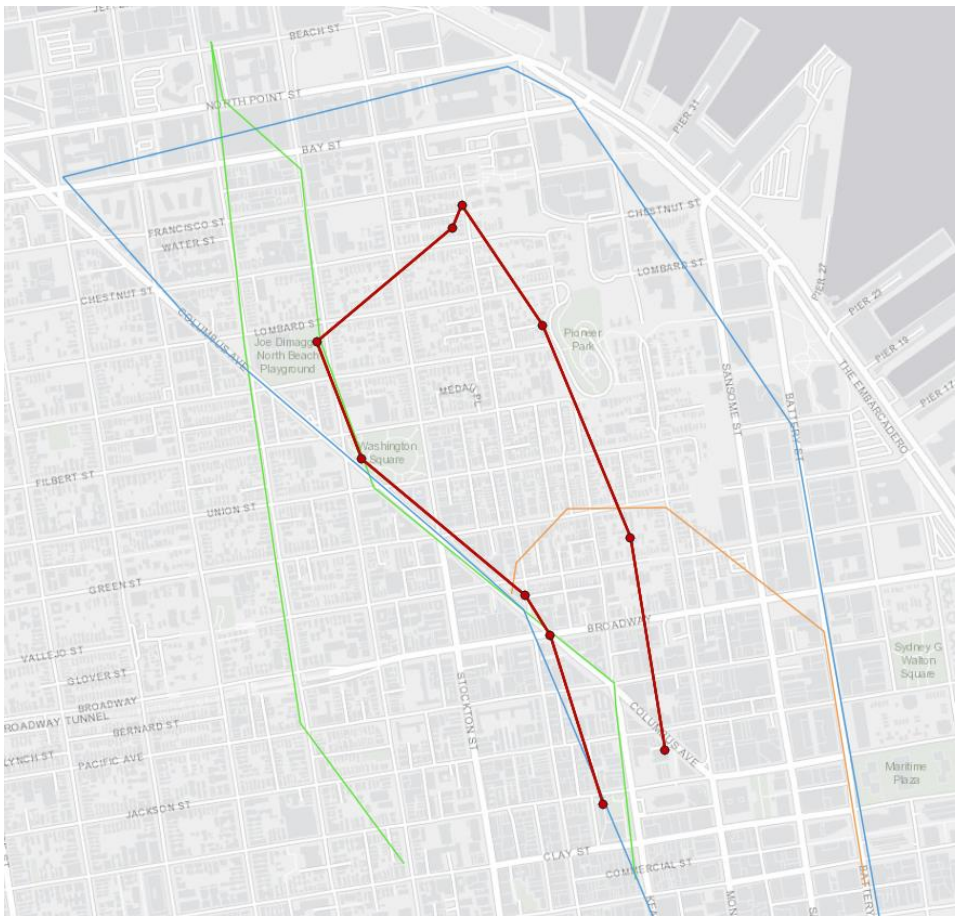
Figure 8 shows an example of the anonymization of trajectories by microaggregation. The anonymized trajectory (red) is the result of the aggregation of k nearest trajectories (depicted in blue, green and orange) included in a cluster, in this case, of size k=3 .
